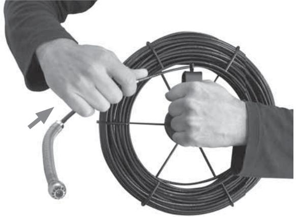
**!** The cable should not be rolled up by turning the reel.
